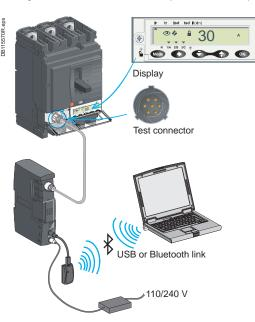
Using the configuration and maintenance module.
